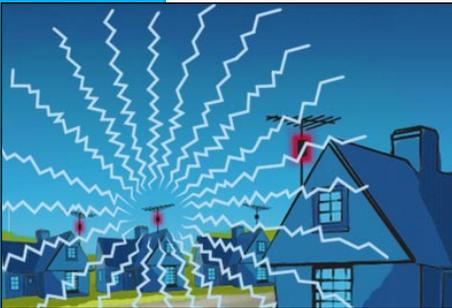
**When a signal booster is faulty, it can cause interference on television receivers in dozens of homes in the neighbourhood. The interference appears in various ways, mainly as more or less stable wavy lines or as horizontal bars. The screen may even go black for a few moments. This type of interference can take many forms.**
