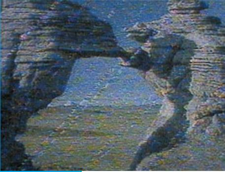
Interference caused by a computer
