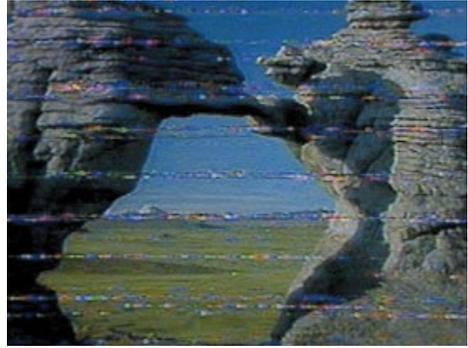
Interference caused by a motor
