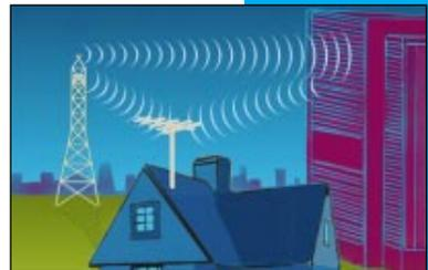
antenna may solve the problem. If reflected signals are coming from behind the television antenna, the ghost image could be reduced or eliminated by using a Yagi antenna or a rear-screen antenna. Poor installation of an antenna can also cause reflected ghost images.
