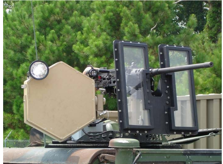
Vehicle mounted Acoustic Hailing Device Official Department of Defense Photos
